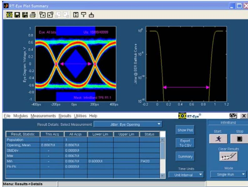
Figure 11 - Results of the Jitter Eye Opening @ 10<sup>-12</sup> BER Measurement
