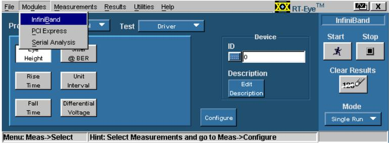
Figure 6 – Choosing the InfiniBand Compliance Module
