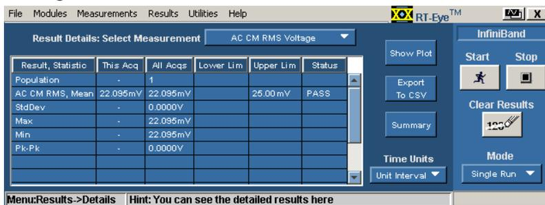
Figure 8 – Result of AC Common Mode Measurement
