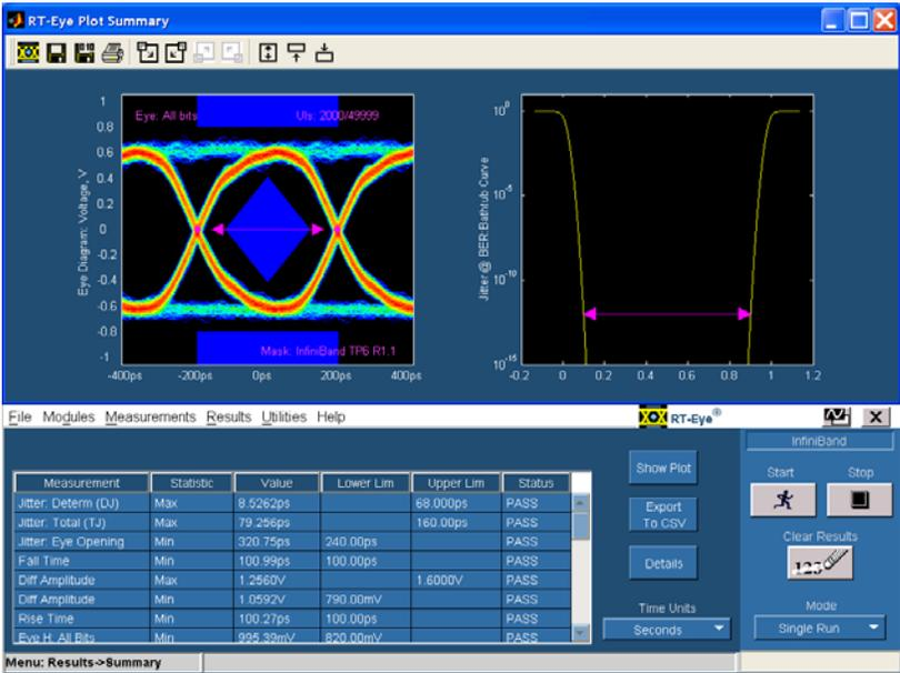
Figure 13 – Combining all measurements into a single test
