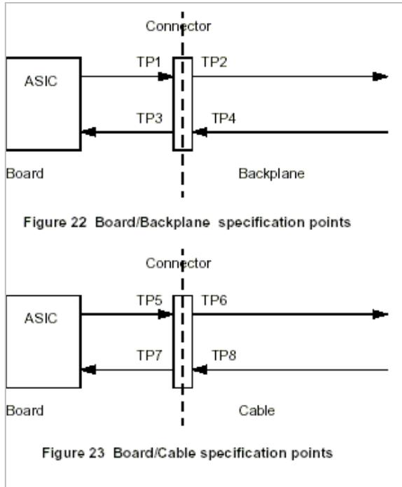
Figure 1 – Compliance Points from the InfiniBand Specification
