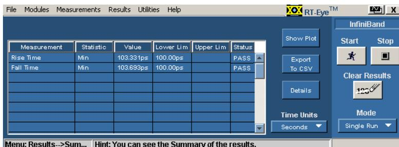
Figure 10 - Results of Transition Time Test
