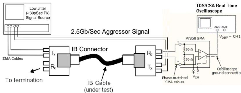
Figure 15 – Test Setup for IB cable testing
