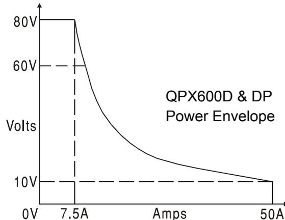
The power envelope is set to give 80V/7.5A and 10V/50A under all supply conditions (both outputs loaded); at lower output voltages the output power is restricted by the 50A current maximum.
