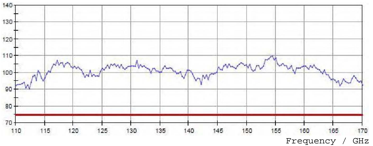
Dynamic range in dB versus frequency of the R&S®ZVA-Z170.
