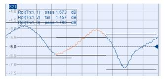
As a consequence of the limit line rules, the limit check will always pass a DUT if no limit lines are defined.
