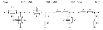
The following networks are composed of a shunt C or L (as seen from the analyzer port), followed by a serial C or L. They are named *Shunt C, Serial C / Shunt C, Serial L / Shunt L, Serial C / Shunt L, Serial L.*
