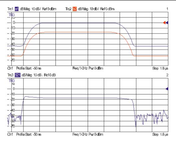
The steepness of the edges of the  $S_{21}$  pulse arises from ratioing (b/a) and does not provide a measure for the rise and fall times of the pulse itself.
