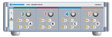
The multiport test set can be configured to provide several channel-specific port groups. The "input" ports (numbered 1 to 4) are connected to the corresponding network analyzer ports. The signal at each "input" port is routed to one of the "output" ports 1 to 4, to be connected to the DUT. Signal routing is channel-dependent, which makes it possible to connect and measure several DUTs in parallel.
