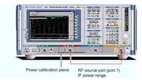
Source power calibration for the LO signal, provided by an external generator. A power sensor is connected to the generator's RF output (red signal). The analyzer controls the generator. The generator's RF source power (red) is calibrated at the selected LO frequency. No RF connection to or from the network analyzer is needed.
