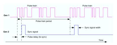
If not specified otherwise, the pulse generator settings are channel-specific.
