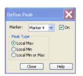
It is possible to select the peak type up to ten times for each trace and assign the selection to the markers no. 1 to 10.
