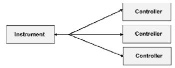
The controllers can lock and unlock the instrument for exclusive access. This regulates access to the instrument of several controllers.
