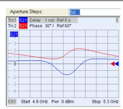
• The 100 MHz aperture in the example above is actually too wide, because the phase shows strong distortions in a frequency interval with a width of approx. 80 MHz. The wide aperture results in a smoothing effect of the delay trace. A reduced aperture of 20 MHz yields a more accurate group delay in the vicinity of the minimum.
