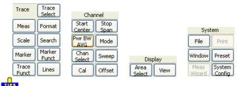
• The hardkey bar provides access to the basic groups of settings with a single mouse click. It is particularly useful if the analyzer is controlled from an external monitor or *Remote Desktop*. Alternatively the settings are accessible from the menus of the menu bar or from the softkey bar.
