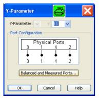
The notation for Y-parameters and the functionality of the *Y-Parameter* dialog is analogous to the definition of S-parameters. The dialog provides the following settings:
