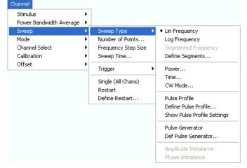
• *Lin. Frequency* is the default sweep type. The stimulus frequency is swept in equidistant steps over the continuous frequency range. In a Cartesian diagram, the x-axis is a linear frequency
