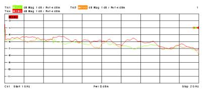
2. In the intermodulation distortion spectrum measurement, the frequency and power of the lower and upper tones is kept constant; the analyzer displays all intermodulation products in the vicinity of the signals up to a selectable order.
