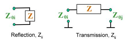
The analyzer converts a **single** measured S-parameter to determine the corresponding converted impedance. As a result, converted Z-parameters cannot completely describe general n-port DUTs:
