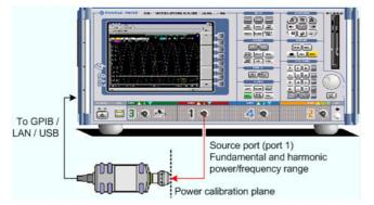
2. Receiver power calibration for the selected harmonic. No external device is needed. The receiver (port 2) is calibrated at the harmonic frequency using the source signal from port 1 (red) calibrated in
