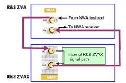
The external connectors are modified if a *High Power Coupler* is fitted at port 1 or port 2 of the Extension Unit. Refer to the R&S ZVAX operating manual for details. Please observe the safety instructions in the R&S ZVAX operating manual.
