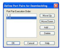
The same physical port(s) may be used repeatedly in different port pairs; it is also possible to repeat the same port pairs. The first pair in the *Embedding* list and the last pair in the *Deembedding* list correspond to the position closest to the DUT. The effect of port pair (de-)embedding depends on the order of the port pairs as shown in the following examples.
