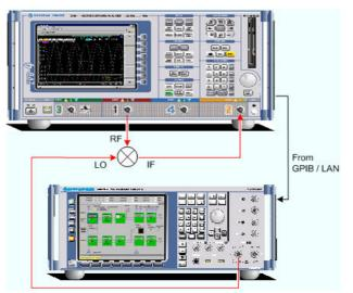
Power calibration: An external generator can provide the reference signal for a source or receiver calibration. A typical example is a receiver power calibration using a measured wave b<sub>1</sub>.
