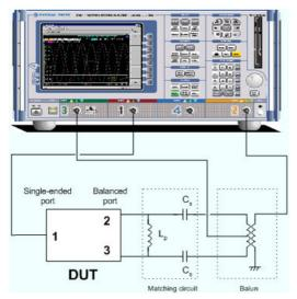
The idea of virtual embedding is to simulate the matching network and avoid using physical circuitry so that the analyzer ports can be directly connected to the input and output ports of the DUT. The matching circuit is taken into account numerically. The analyzer measures the DUT alone but provides the characteristics of the DUT, including the desired matching circuit. This method provides a number of advantages:
