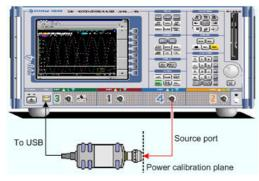
Configured external power meters can be selected as additional receivers in the *Port Configuration* and in the power calibration dialogs.
