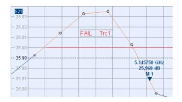
Remote control: CALCulate<Chn>:LIMit:STATe ON | OFF CALCulate<Chn>:LIMit:LOWer:STATe ON | OFF
