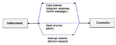
The number of controllers that can address an instrument is practically unlimited in the network. In the instrument, the individual controllers are clearly distinguished. This distinction continues up to the application level in the controller, i.e. two applications on a computer are identified by the instrument as two different controllers.
