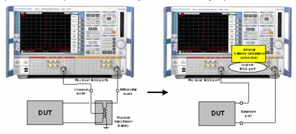
Unbalance-balance conversion avoids the disadvantages of real transformers:
