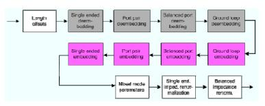
This means that the real networks are removed before virtual networks are added. For a single balanced port with all single ended and balanced port (de-)embedding networks enabled, the 4 (de-)embedding steps are carried out in the following order:
