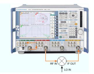
Test setup 2: Coupler used as an internal combiner
