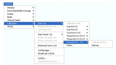
Four-port calibrations can be performed automatically or manually.
