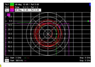
A double-click into any point in the diagram area is equivalent to the *Maximize* function. To view all traces in a common, maximized diagram area, select *Overlay all*.
