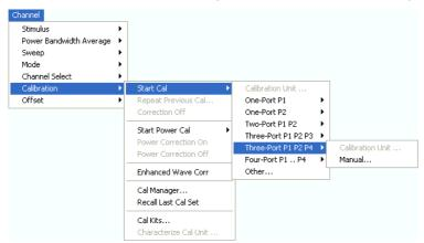
Three-port calibrations can be performed automatically or manually.
