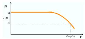
The compression point is a measure for the upper edge of the linearity range of a DUT. It is close to the highest input signal level for which the DUT shows a linear response  $(|a_n| \longrightarrow x^*|a_n| \implies |b_n| \longrightarrow x^*|b_n|$ , so that the magnitude of all S-parameters remains constant).
