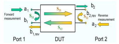
The S-parameters are the basic measured quantities of a network analyzer. They describe how the DUT modifies a signal that is transmitted or reflected in forward or reverse direction. S-parameters are expressed as  $S_{\text{out}>(in>)}$ , where <out> and <in> denote the output and input port numbers of the DUT.
