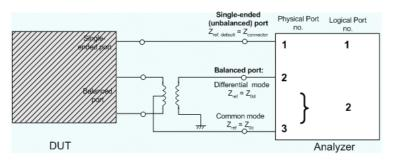
The default values for the balanced port reference impedances are derived from the default reference impedance of the physical analyzer ports ( $Z_0 = 50 > \Omega$ ):
