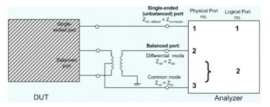
The default values for the balanced port reference impedances are derived from the (real) default reference impedance of the physical analyzer ports ( $Z_0 = 50 > \Omega$ ):
