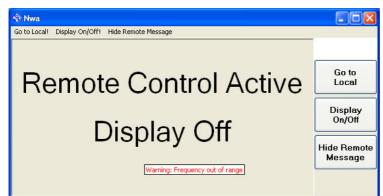
The softkeys in the remote screen are used to modify or quit the remote state:
