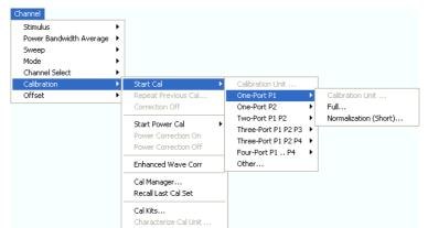
One-port calibrations can be performed automatically or manually.
