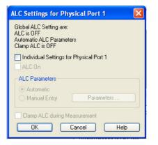
Remote control: SOURce<Ch>:POWer<Pt>:ALC:CONTrol SOURce<Ch>:POWer<Pt>:ALC[:STATe] SOURce<Ch>:POWer<Pt>:ALC:PIParameter
