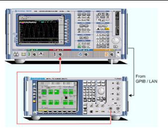
Configured external generators can be selected as additional sources in the *More Wave Quantities, More Ratios, Port Configuration,* and in the power calibration dialogs.
