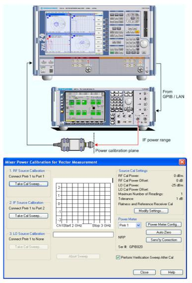
• *Take Cal Sweep* in the three numbered panels starts the calibration sweeps for the RF source, IF source, and the LO source, respectively. The measured power is shown in the diagram in the center of the dialog and the sweep progress in the progress bar below.
