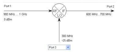
Calibration kits do not contain frequency-converting two-port standards so that any system error correction is performed at equal source and receiver frequencies. However, if a scalar mixer measurement is active, the analyzer automatically performs the system error correction in both the RF and the IF frequency range. The number of points for the calibration sweep is doubled. In the *Calibration Manager* dialog, the calibrated frequency range is referred to as a "Segmented Grid".
