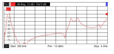
Remote control: [SENSe<Ch>:]SWEep:TPYE LINear [SENSe<Chn>:]FUNCtion[:ON] "XFRequency:..."
