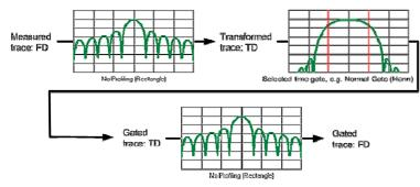
The shape, width and position of the time gate affect the gated frequency domain trace. The window type selection in the *Define Transform* dialog is ignored. The selected window is used again when the TD trace is displayed (*Time Domain: On*).
