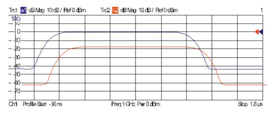
The magnitude of the S-parameter  $S_{21}$  is distorted at the beginning and at the end of the pulses because the analyzer divides the two wave quantities at equal times.
