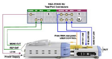
The external test sets enable a frequency range between 10 MHz and 80 GHz. The analyzer combines two different measurement methods to achieve this extended range.
