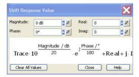
The units of the constants are adjusted to the format of the active trace. Setting all values to zero (*Clear All Values*) restores the original trace.
