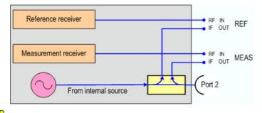
The signal description above with the swept RF signal and the LO signal at a fixed frequency corresponds to the default configuration. In the *Set Frequencies* dialog, you can select any of the signals as a *Sweep/CW* signal. You can set the frequency range of this signal via *Start/Stop or CW Frequency*. A second signal is at a *Fixed* frequency, and the third at the calculated sum or difference frequency (*Auto*).
