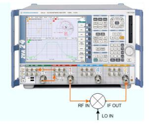
The *Define Mixer Measurement* dialog can be accessed from the intermodulation distortion measurement dialog. You can also use the *Port Configuration* dialog to configure an arbitrary frequency-converting measurement.
