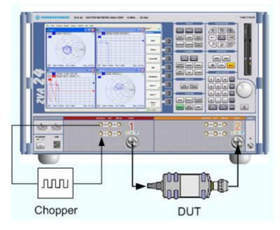
The analyzer measures the pulse profile of the reflected and transmitted waves, i.e. the magnitudes of the wave quantities  $a_1$  and  $b_2$  vs. time and calculates the forward transmission coefficient  $S_{21}$ .
