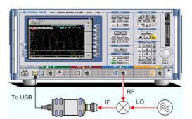
• Power calibration: An external power meter can measure the exact signal power at an arbitrary point in the test setup (reference plane) and thus provide the reference values for a power calibration. A typical example is a source power calibration for an arbitrary analyzer port.
