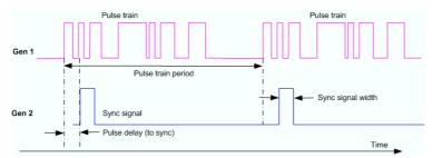
If not specified otherwise, the pulse generator settings are channel-specific.
