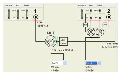
The mixer vector calibration corresponds to a 2-port UOSM calibration where the unknown through standard is replaced by an unknown calibration mixer. In analogy to the unknown through standard used for UOSM calibration, the calibration mixer must be reciprocal ( $S_{21} = S_{12}$ ).
