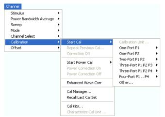
The calibration types depend on the number of test ports of the analyzer. For a four-port unit:
