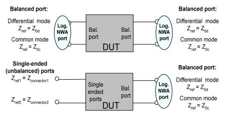
A balanced port configuration is defined by simply selecting the pairs of physical ports that are combined to form balanced ports and defining the two reference impedances for the differential and common mode at each balanced port. All this is done in a single dialog; refer to the help system for details and measurement examples. The most commonly used balanced port configurations and impedances are predefined and can be selected in the *Measurement Wizard*.
