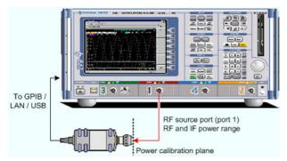
2. Receiver power calibration for the IF signal. No external device is needed. The receiver (port 2) is calibrated in the IF frequency range using the source signal from port 1 (red) calibrated in the first step.
