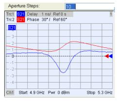
The following table lists "optimum" apertures  $\Delta f = 0.3 / \tau_{g,meas}$  together with sample analyzer settings for a frequency sweep with 201 sweep points. Notice that the sweep span must be reduced or the number of frequency points increased to obtain small apertures.
