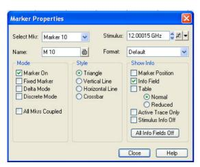
In the left part the dialog contains four input fields and drop-down lists to select a marker and define the basic properties of a selected marker which is switched on in the *Mode* panel.
