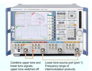
The calibration steps for the other test setups are analogous. Refer to the indications in the power calibration dialog for a correct connection of the power meter and the receive port.
