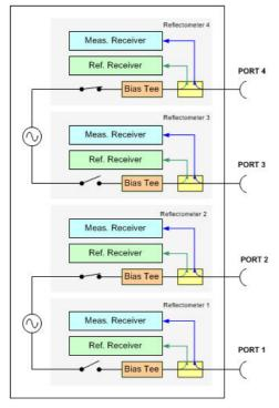
If the RF signal is simultaneously fed to two coupled ports (i.e. if *Gen* is switched on so that at least one signal source is permanent), the port frequencies must be the same. For normal measurements (*Gen*
