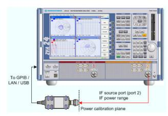
Source power calibration for the LO signal, provided by an external generator. A power sensor is connected to the generator's RF output (red signal). The analyzer controls the generator, its RF power (red) is calibrated at the selected IF frequency. No RF connection to or from the network analyzer is needed.
