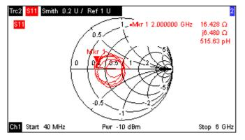
A comparison of the Smith chart, the inverted Smith chart and the polar diagram reveals many similarities between the two representations. In fact the shape of a trace does not change at all if the display format is switched from *Polar* to *Smith* or *Inverted Smith* – the analyzer simply replaces the underlying grid and the default marker format.
