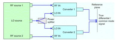
Depending on the network analyzer type and the number of independent sources available, different test setups are possible.
