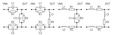
The following networks are composed of a shunt C or L (as seen from the analyzer test port), followed by two serial Cs or Ls. They are named *Shunt C, Serial Cs / Shunt C, Serial Ls / Shunt L, Serial Cs / Shunt L, Serial Ls.*
