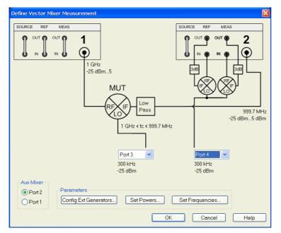
In the upper part the *Define Mixer Measurement* dialog shows a diagram with the test setup for vector mixer measurements. Below the dialog provides the following control elements:
