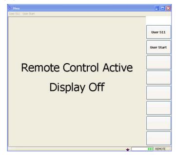
Pressing a user softkey or clicking the corresponding command across the top of the remote screen executes the assigned functionality.
