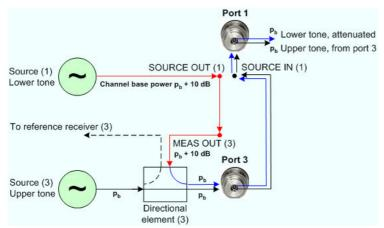
Larger *Port Power Offset* values (and hence smaller compensating *Cal Power Offset* values) may be required e.g. to account for an additional cable loss in the test setup. The maximum source power (depending on the analyzer model and the frequency; see data sheet) must not be exceeded. If necessary, reduce the channel base power (and thus the *Cal Power*).
