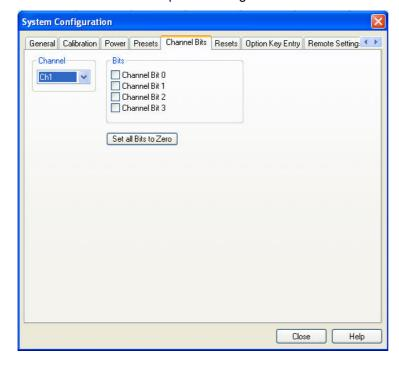
**Remote control** CONTrol:AUXiliary:C[:DATA] (for Channel Bits): OUTPut<Ch>:UPORt[:VALue]
