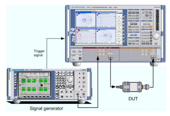
The analyzer measures the pulse profile, i.e. the magnitude of the received wave quantity (typically  $b_2$ ) vs. time.
