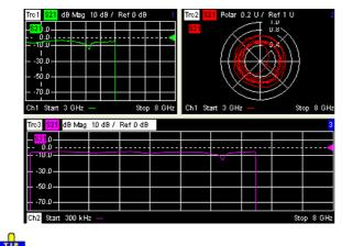
**-**To vary the size and position of the diagram areas, drag and drop the separating frames, use the Split Manager or the functions of the Window menu.
