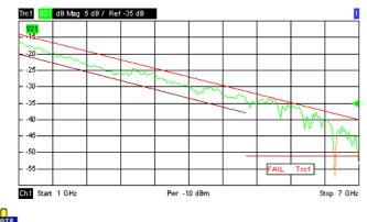
Limit check and display of the limit lines are independent of each other: With disabled limit check, the limit line can still be displayed.
