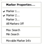
*Movable Marker Info* allows the marker info field to be placed to any position in the diagram area. The remaining settings correspond to the most common commands in the *Trace – Marker* and *Trace – Search* menus.
