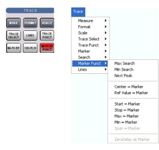
The functions in the upper section are also provided in the Search submenu:
