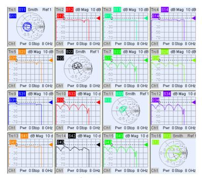
A n-port analyzer provides  $n^2$  independent S-parameters  $S_{\text{out}>\text{sin}}$ . If a balanced port configuration is defined, the normal S-parameters are replaced by mixed mode parameters.
