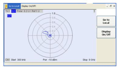
Switching on the display is ideal for program test purposes but tends to slow down the measurement. Therefore it is recommended to switch off the display in real measurement applications where a tested program script is to be executed repeatedly.
