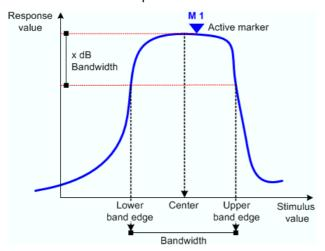
In contrast to a *Bandpass Search Ref to Max,* the *Bandpass Search Ref to Marker* does not change the position of the active markers. The *Loss* is the response value at the marker position; the bandfilter
