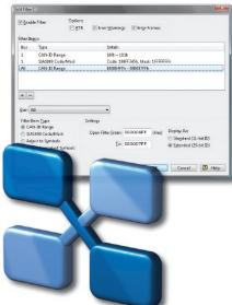
PCAN-Explorer is an universal tool for monitoring data traffic on a CAN network. For easy and clear allocation of the individual messages, these can be identified as so-called symbols. The integrated VBScript support allows the creation of macros to automate complex tasks. The integrated data logger means that the data traffic of a bus can be recorded, analyzed, and stored. PCAN-Explorer is designed as automation server and can therefore be remote controlled through scripts.
