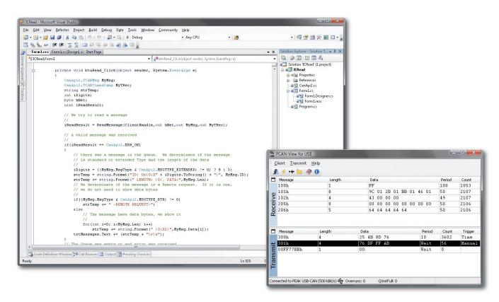
PCAN is a flexible system for planning, developing and applying CAN networks. Windows Kernel mode ring-0 drivers are the basis for communication between PCs and external hardware via a CAN bus. These form the core of a complete CAN network environment on a PC running Windows.
