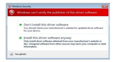
Once the driver is loaded on the PC a virtual COM port will be established each time the instrument is powered up and connected to the PC via USB. The virtual COM port will disappear if either of these cease to be true.
