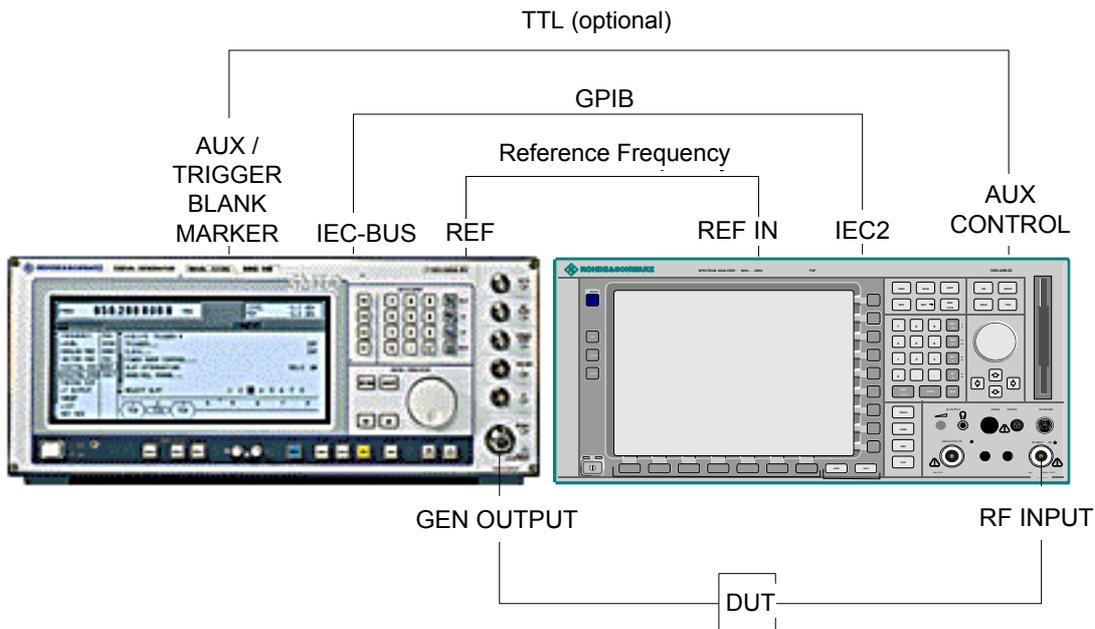
The generator is controlled via the – optional – second GPIB interface of the R&S FSP (= IEC2, supplied together with the option). With some Rohde & Schwarz generators, it is also controlled via the TTL synchronization interface that is contained in the AUX CONTROL interface of the R&S FSP.
