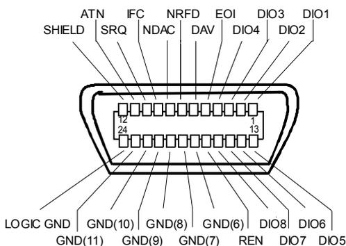
Fig. 1-9 Pin assignment of the second IEC interface
