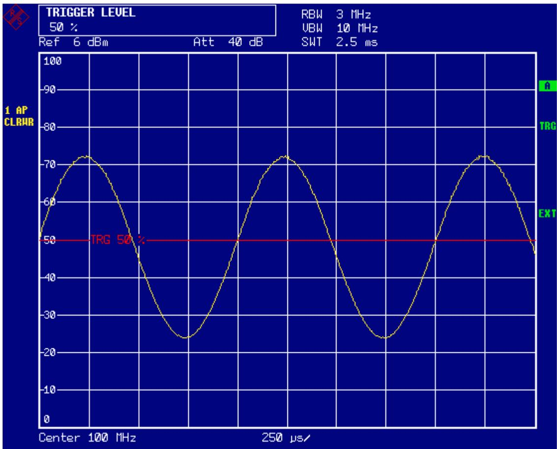
Fig. 5-13 Measurement of the AF signal of a carrier that is AM-modulated with 1 kHz
