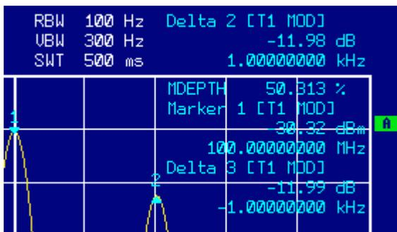
Fig. 5-7 Measurement of the AM modulation depth. The modulation depth shown is MDEPTH. The frequency of the AF signal can be obtained from the frequency display of the delta marker.
