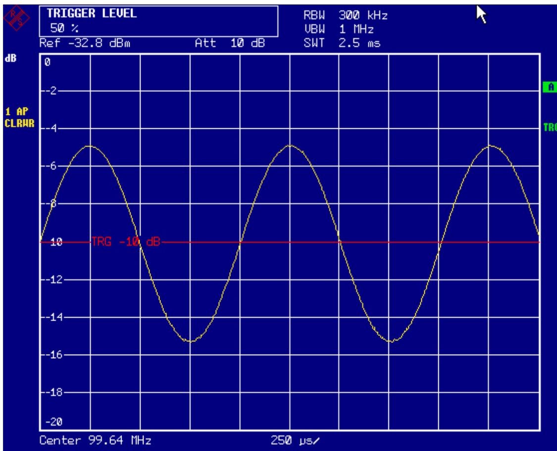
Fig. 5-15 Display of the demodulated FM signal
