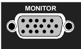
After connecting the external monitor, restart the instrument to detect the monitor. The measurement display will then appear on both the external screen and on the instrument. No further settings are necessary.
