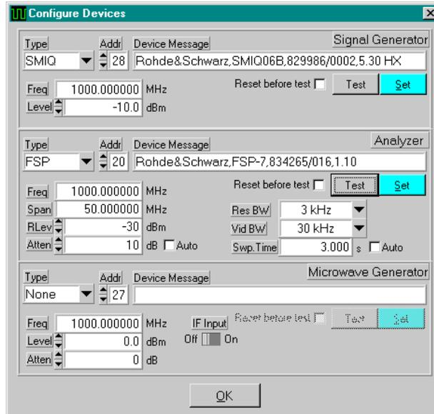
Fig. 22 Device Configuration
