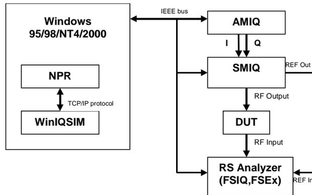
Fig. 1 Connecting Instruments
