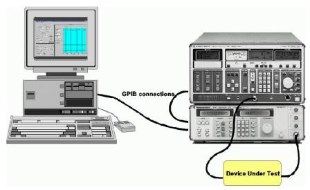
Fig. 1 Connecting computer to instruments
