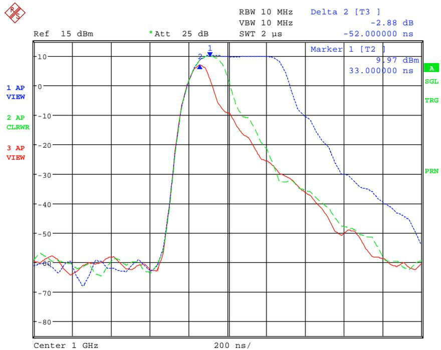
Fig 4: Peak power reading at the top of the pulse.
