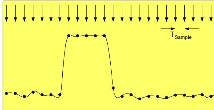
Fig 11 Sampling of a pulse signals in time domain.
