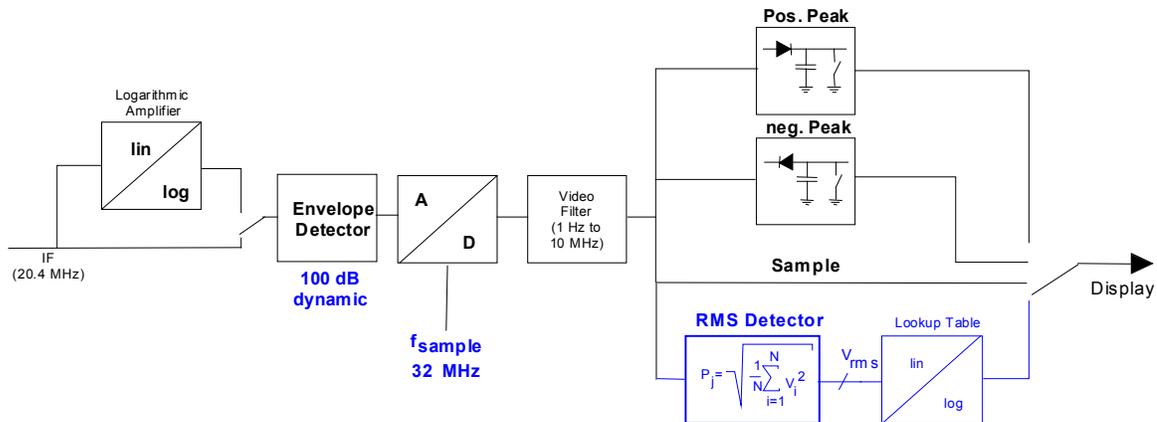
Fig. 2 Block diagram of the detector implementation.
