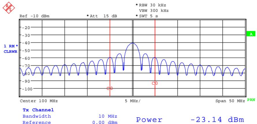
Fig 6 Channel power measurement with 10 MHz channel bandwidth.
