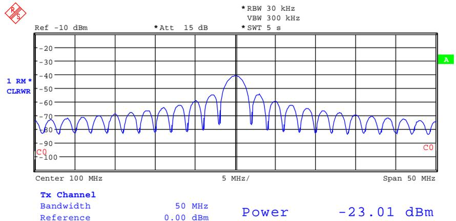
Fig 7 Channel power measurement with 50 MHz channel bandwidth.
