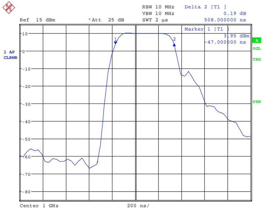
Fig 5 Pulse width reading with delta markers.
