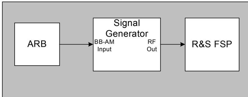
Fig. 3 Test setup for the measurement examples
