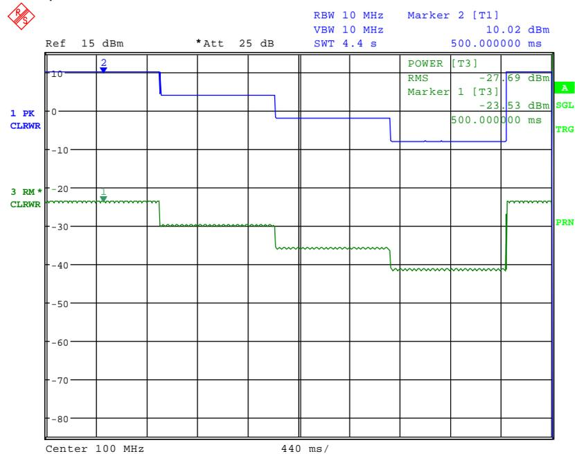
Fig 9 Summary power with wrong measurement time.
