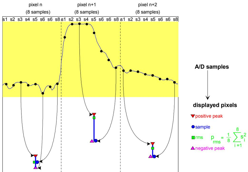
Fig. 1 Symbolic graph of data reduction on the display.
