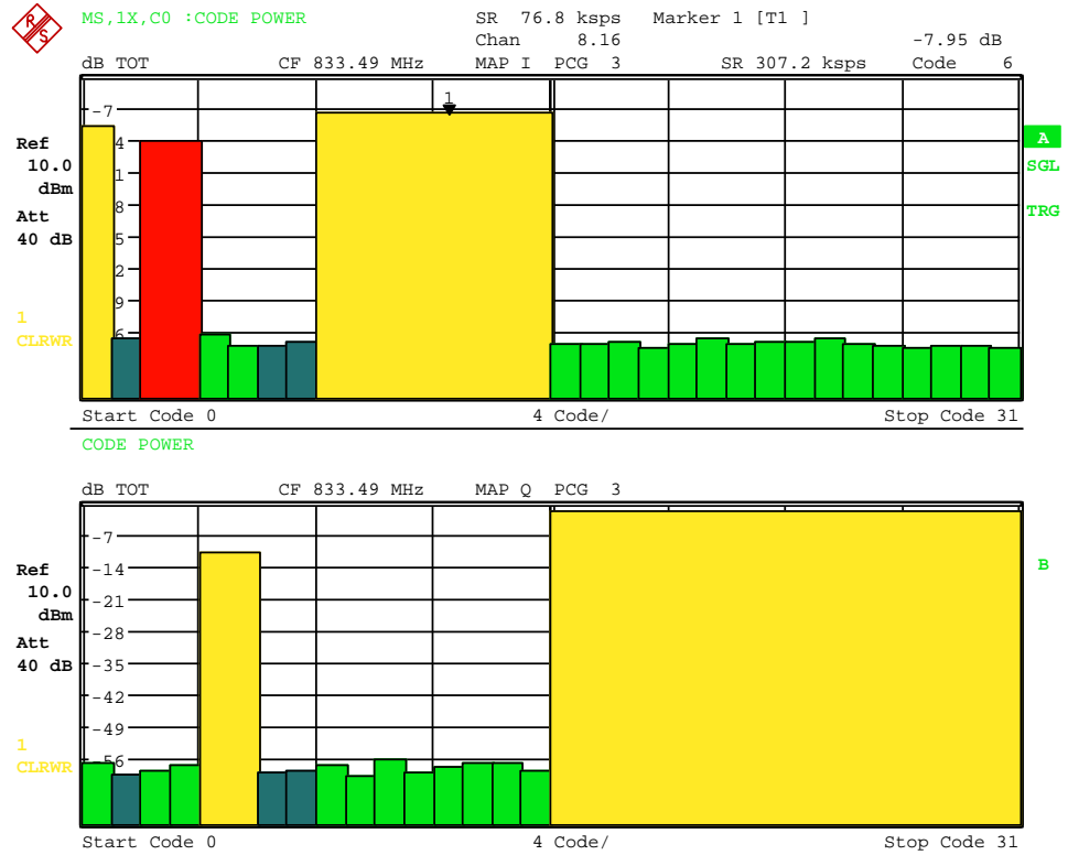
Fig. 6-9 CDP diagram in BitReverse order in overview mode
