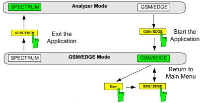
Figure 2-1 Starting and exiting the application
