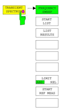
Press the *TRANSIENT SPECTRUM* softkey to call the submenu for measuring the spectrum due to transients. In the default setting, the SPECTRUM ANALYZER measures the spectrum due to transients in the frequency domain (*FREQUENCY SWEEP*).
