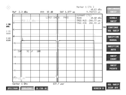
Figure 2-11 PVT measurement – TOP HIGH RESOLUTION
