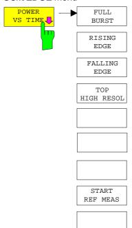
Press the *POWER VS TIME* softkey to start measurement of carrier power versus time and open a submenu for configuring the display. The power of the burst is also measured as centered relative to the midamble and displayed.
