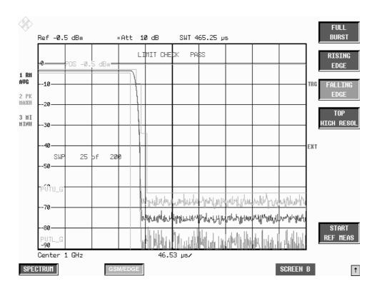
Figure 2-10 PVT measurement – FALLING EDGE
