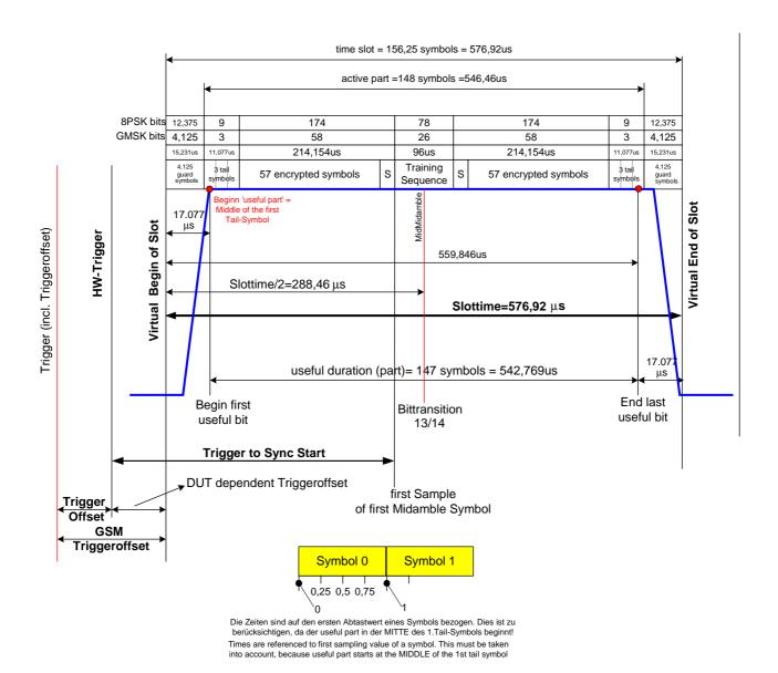
Figure 1-4 Trigger and time references
