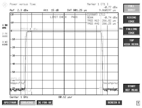
Figure 2-7 PVT single slot measurement – FULL BURST
