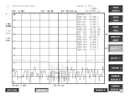
Figure 2-4 Measurement of Modulation Accuracy
