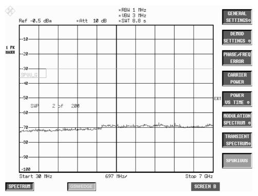
Figure 2-18 Measurement of spurious
