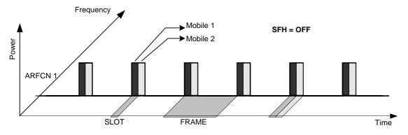
Mobile 1 transmitting on same frequency, mobile 2 transmitting on different frequencies
