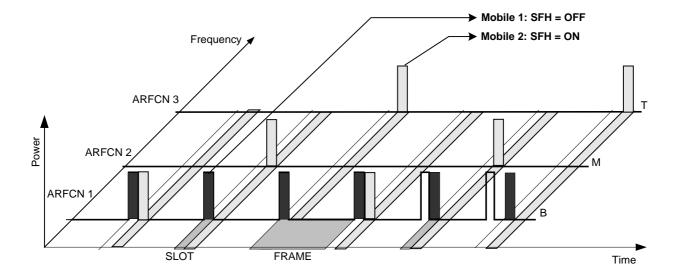
Figure 1-1 Data transmission in GSM network - T&FDMA communication
