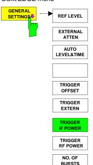
Pressing the *GENERAL SETTINGS* softkey opens a submenu for setting the major parameters of the GSM/EDGE base and mobile station tests application.
