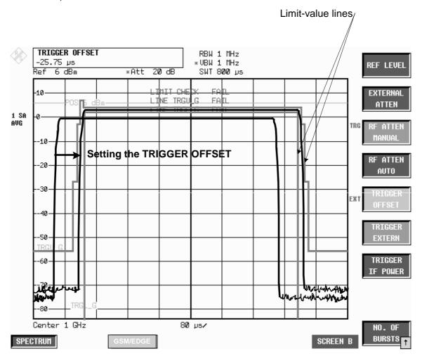
Figure 1-3 Trigger setting in GENERAL SETTINGS menu
