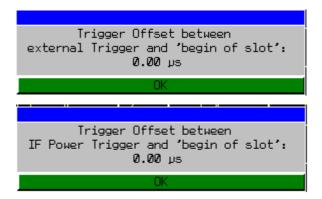
**Note:** The values determined here for the GSM trigger offset must be specified in remote-control mode for correct synchronization with the
