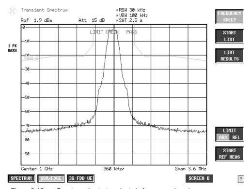
Figure 2-15 Spectrum due to transients in frequency domain
