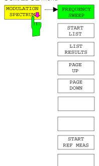
The MODULATION SPECTRUM softkey calls the submenu for measuring the spectrum due to modulation. In the default setting, the spectrum analyzer measures the spectrum due to modulation in the frequency domain (FREQUENCY SWEEP).
