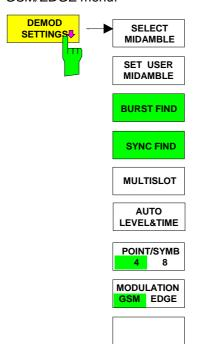
Pressing the *DEMOD SETTINGS* softkey opens a submenu for setting the major parameters of the demodulator in the GSM/EDGE application.
