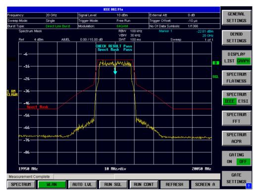
Fig. 2-20 EEE 802.11a Spectrum Mask Results
