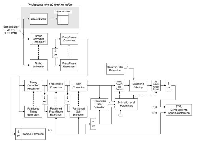
Fig. 3-2 Signal processing of the IEEE802.11b application
