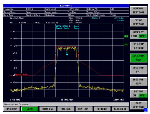
Fig. 2-21 EEE 802.11b/j Spectrum Mask Results
