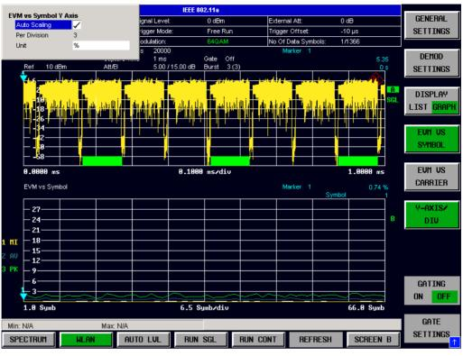
Fig. 2-9 EVM Vs Symbol - Y-Axis Scaling
