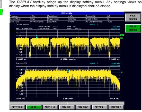
The layout of the display can be controlled using the display menu
