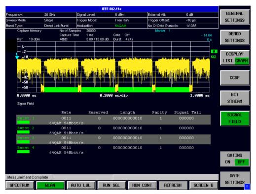
Fig. 2-18 Bit-Stream Signal Field Results
