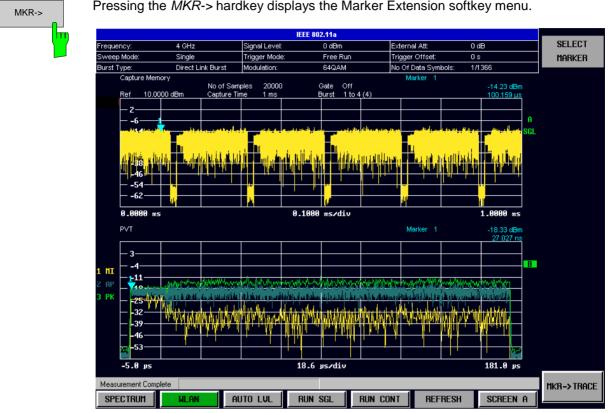
Pressing the *MKR->* hardkey displays the Marker Extension softkey menu.
