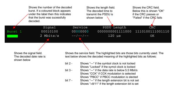
When no other dialogs are on display the results can be scrolled through using the cursor keys or scroll wheel. This measurement is only available when the IEEE 802.11b standard is selected
