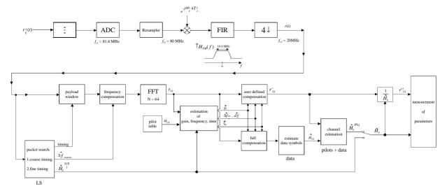
Fig. 3-1 Signal processing of the IEEE802.11a application
