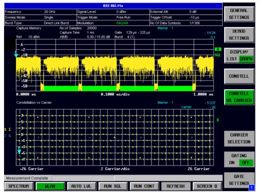
Fig. 2-14 Constellation Vs Carrier Results
