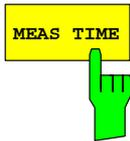
The *MEAS TIME* softkey opens a list in which the measurement can be set. Results are more stable with longer measurement times, particularly if signals with lower power are measured.
