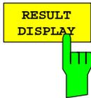
The *RESULT DISPLAY* softkey switches the result display of the power measurement on or off. If the display is switched off, the measured power appears in the Marker Info field.
