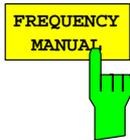
The **FREQUENCY MANUAL** softkey opens the data entry field for the frequency of the signal to be measured.
