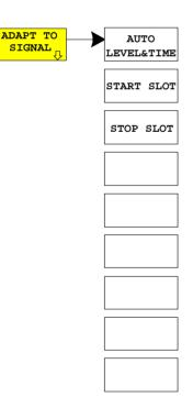
The *ADAPT TO SIGNAL* softkey opens a submenu for matching the reference level of the analyzer and configuration of gated sweep mode.
