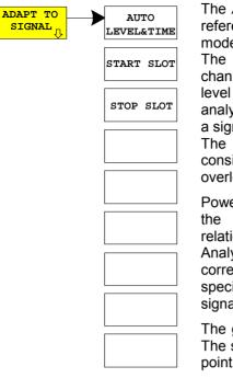
The *ADAPT TO SIGNAL softkey* opens a submenu for matching the reference level of the analyzer and configuration of the gated sweep mode.
