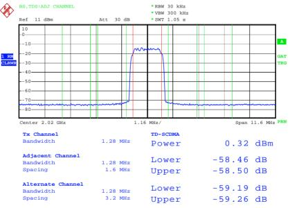
Fig. 5-2 Measuring adjacent channel power
