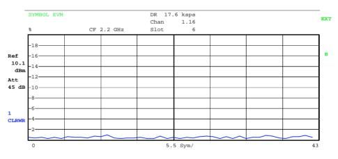
Fig. 5-19 Error vector magnitude for one channel of slot
