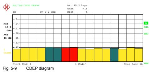
By entering a channel number (see *SELECT CHANNEL* softkey), you can select a channel for more detailed display. The codes of this channel are shown in red.
