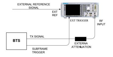
Fig. 3-1 BTS test setup
