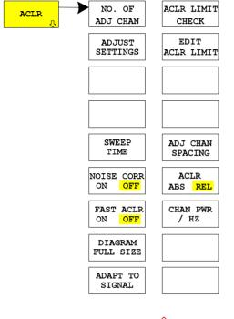
The *ACLR* (adjacent channel leakage power ratio) softkey activates measurement of adjacent channel power. Settings and limits are taken from the ACLR measurement defined in TD-SCDMA specifications.
