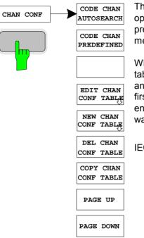
The *CHAN CONF* hotkey opens a submenu with configuration options for the channel search. In this submenu you can select predefined channel tables that are then taken as a basis for measurements by the code domain analyzer.
