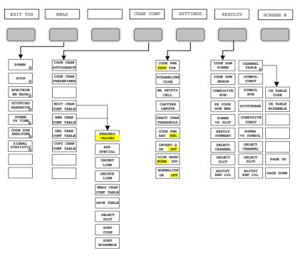
Fig. 4-2 Overview of menus in Application Firmware R&S FS-K76
