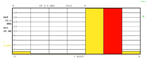
Fig. 5-11 Composite EVM diagram with unrecognized channels
