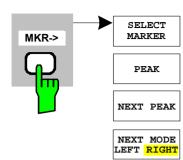
The  $MKR \rightarrow$  key opens a submenu for marker functions:
