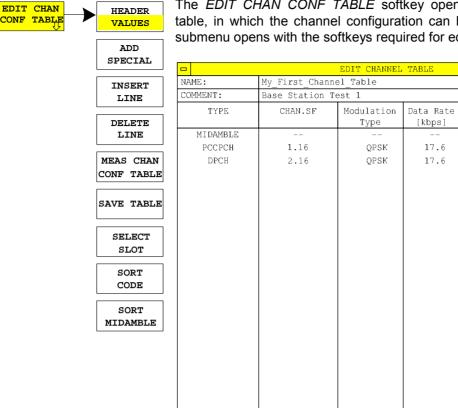
The EDIT CHAN CONF TABLE softkey opens the selected channel table, in which the channel configuration can be edited. In addition, a submenu opens with the softkeys required for editing the channel table.
