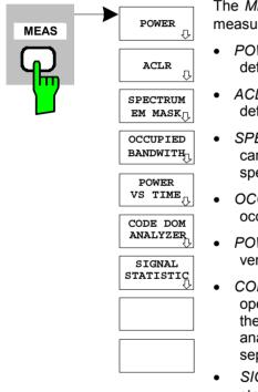
The *MEAS* hotkey or the *MEAS* key opens a submenu for selecting measurements:
