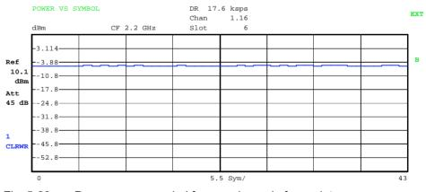
Fig. 5-23 Power versus symbol for one channel of one slot
