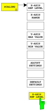
The *SCALING* softkey opens a menu on which the scaling parameters for the X-axis and the Y-axis can be modified.
