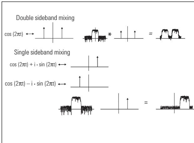
**Figure 19. Using a complex sinusoid to achieve one-sided frequency translation**
