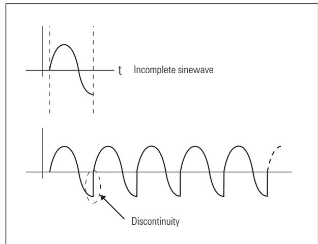
**Figure 15. Demonstration of the spectral effect of adding a discontinuity to a sinewave**
