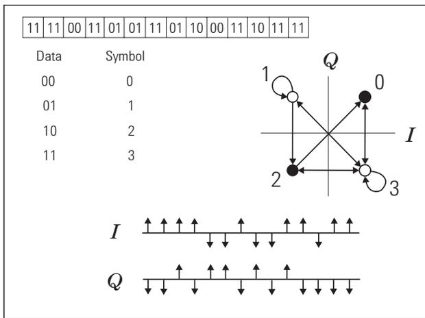
Figure 9. Building QPSK symbols from binary data
