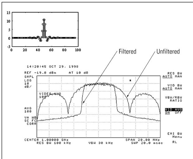
**Figure 10. Impulse response and frequency response of root Nyquist filter**
