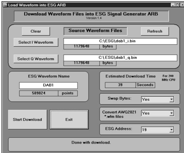
**Figure 14. Windows-based download utility for Agilent ESG arbitrary waveform files**
