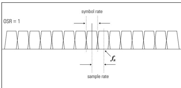
Figure 11. Frequency response of a signal sampled at the Nyquist rate
