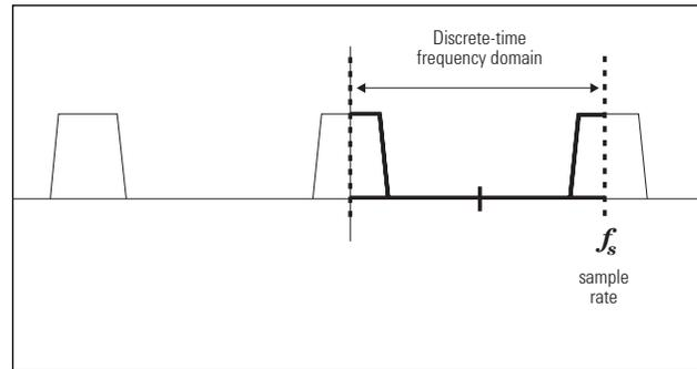
**Figure 24. Correspondence between discrete-time frequency and continuous time frequency**
