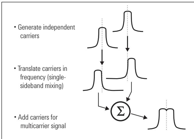
Figure 18. Multicarrier signal generation process
