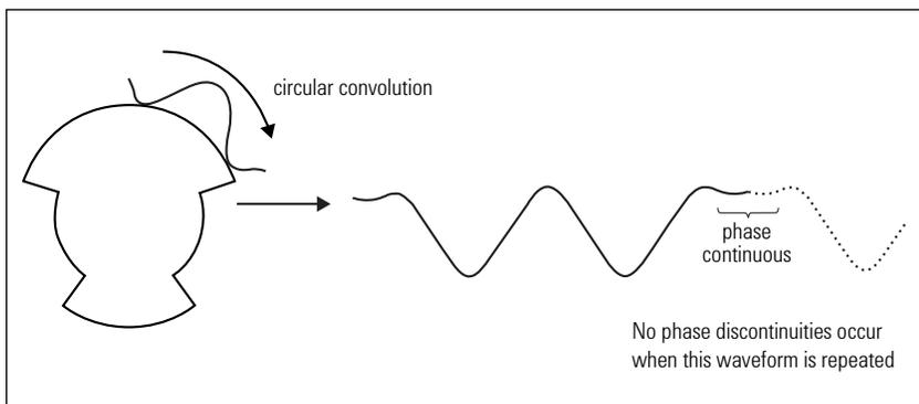
**Figure 17. Using circular convolution to eliminate filter delay and phase discontinuities for FIR filtering**
