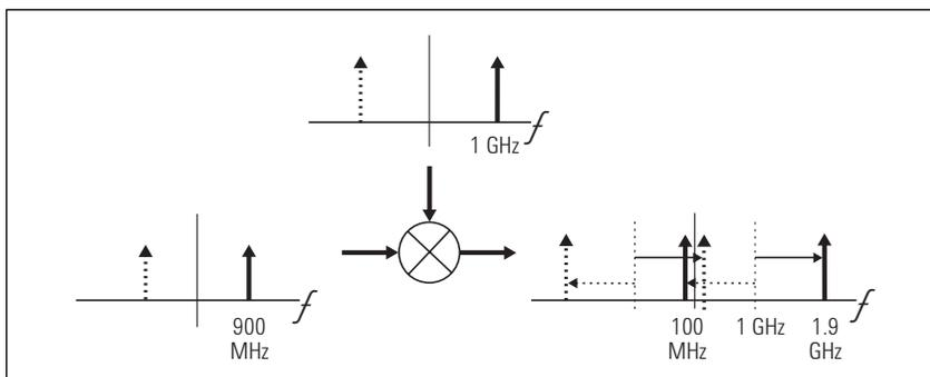
**Figure 3. Spectrum “reversal” after heterodyning a complex-modulated signal to achieve a 100 MHz carrier**
