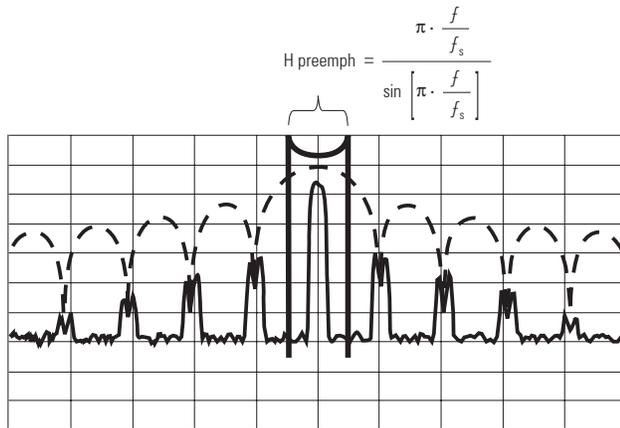
**Figure 23. Preemphasis filter used to cancel effects of sample-and-hold DAC rolloff for wide baseband signals**
