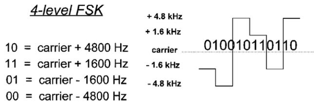
Figure 9. 4-level FSK FLEX™ signaling
