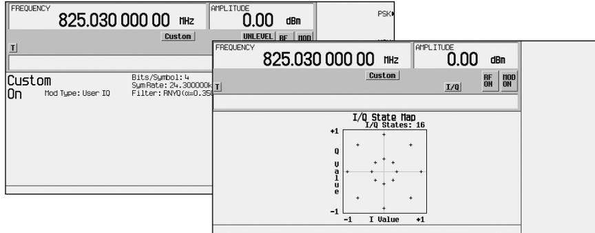
Figure 13. Custom modulation and I/Q display
