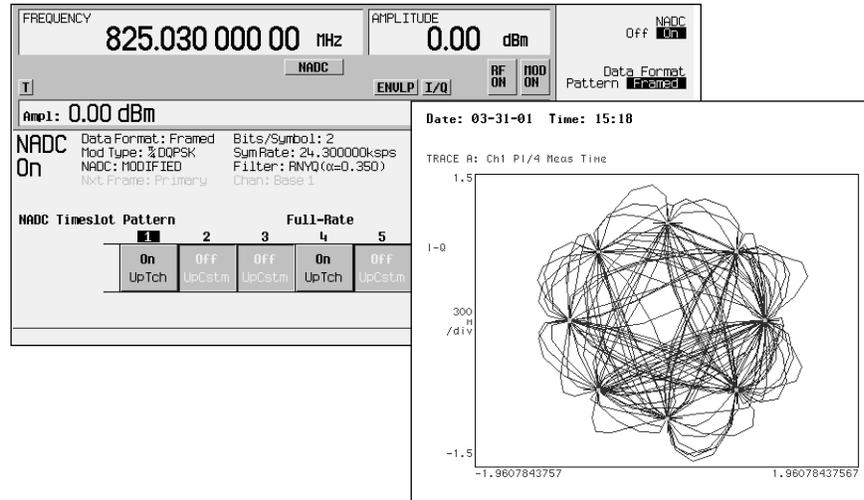
Figure 4. NADC setup and resulting signal
