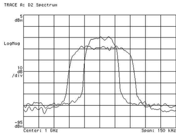
**Figure 28. Determining filter bandwidth**
