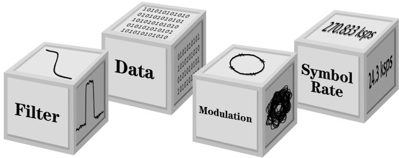
Figure 6. Building blocks of a digitally modulated signal
