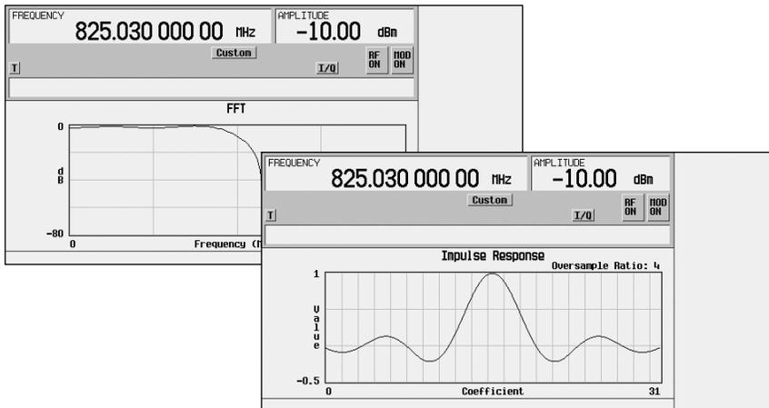
Figure 26. Filter response and FFT of custom FIR filter
