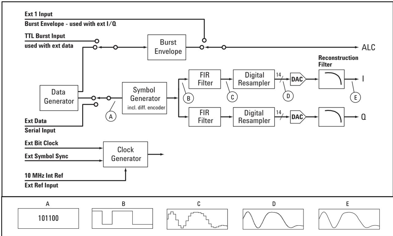
Figure 2. Real-time I/Q baseband generator block diagram
