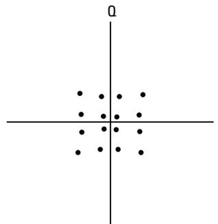
Figure 20. 16QAM distortion
