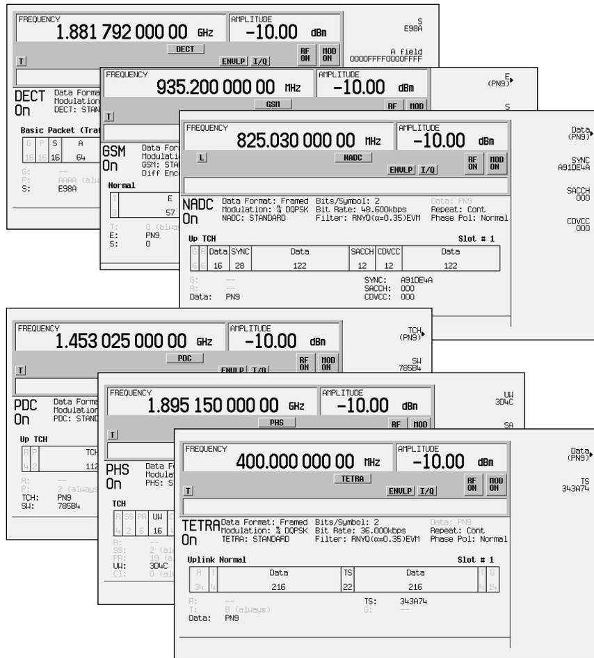
**Figure 3. Supported TDMA standards with protocols**
