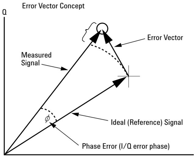
Figure 10. The I/Q diagram
