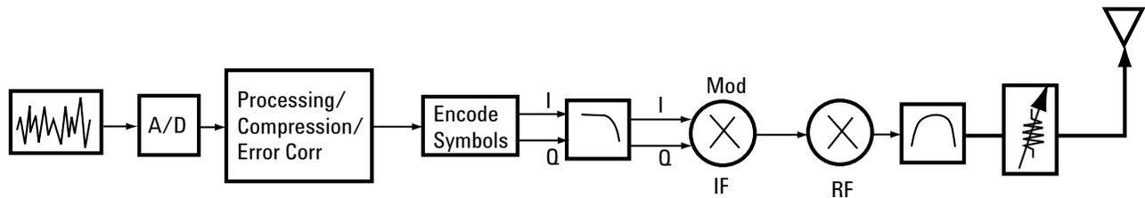
Figure 1. Engineering the signal path using a signal generator
