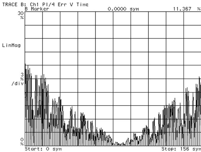
**Figure 29. Effects of 0.008 symbol/symbol clock drift**
