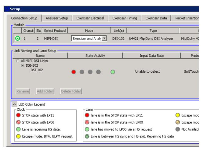
You specify the connection details on the basis of the stimulus/analysis functions that you want the U4421A module to perform. The connection setup details that you specify in this tab tells the Logic and Protocol Analyzer software how the U4421A module is connected to the DUT in terms such as the connection mode, probing option used and the link
