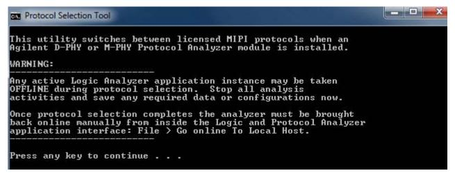
3 Specify the slot number in which you installed the U4421A module for which you want to select the protocol. Press <Enter>.
