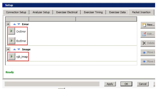
g Click the button displayed for a command button to dynamically insert the packets that you associated to that command button
