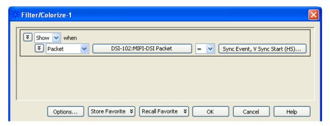
The following screen displays the filtered D-PHY data on the basis of the type of packet. Only the *V Sync Start (HS)* packets are displayed after filtering.
