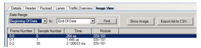
All data formats in the CSI-2 and DSI specifications are supported for image construction in the Image View tab.
