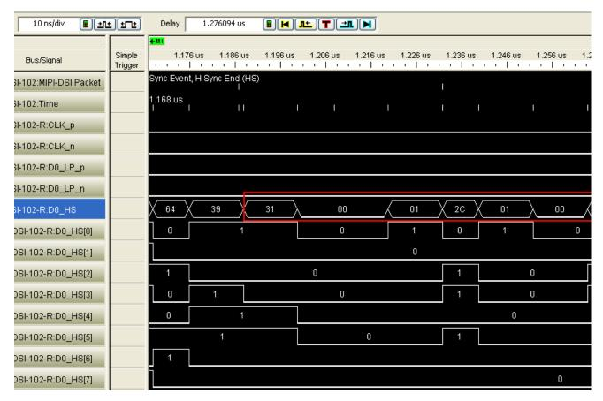
You can correlate the data displayed in the waveform with the relevant packet(s) in the Protocol Viewer. The following screen displays the correlated packet and its data across lanes for the signal data highlighted in the above screen.
