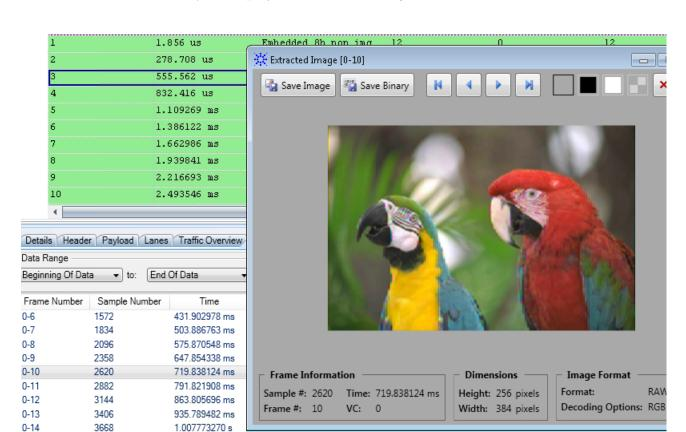
A sample image constructed from the start of frame 10 (sample number 2620) is displayed in the following screen.
