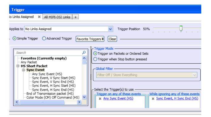
The following trigger setup triggers the U4421A module on the transmission of a packet with any of the errors included as trigger events.
