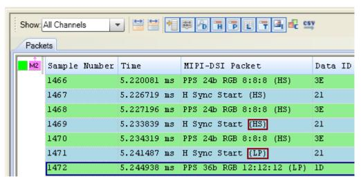
You can also view this information for a packet in the Details tab in the lower pane of the Protocol Viewer. The Details tab shows the **State of Line** and **Lane Mode** applicable for the D-PHY packet selected in the upper pane.
