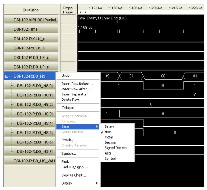
On selecting Binary as the Base unit, the display is changed to binary data values.
