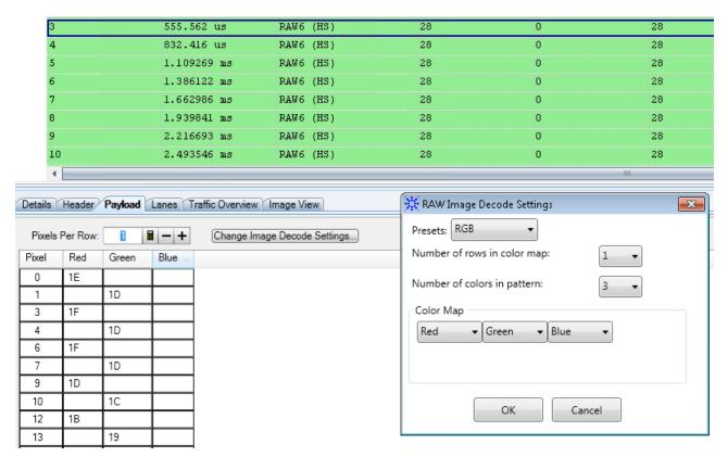
For RAW formats, a number of preset options such as RGB, YMC, CMY, and Bayer decoding are available in the Raw Image Decode Settings dialog box. Based on the decode settings that you select in this dialog box, the image's payload data is recalculated in the Payload tab. The changed settings are also applicable while extracting an image in the **Image View** tab.
