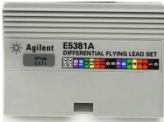
Figure 7 Color coding for flying lead cables
