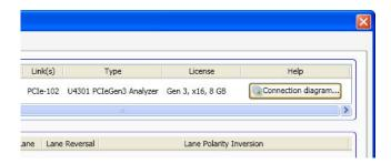
**b** Use the Connection Diagram dialog to verify that your connection setup specification matches the actual device under test connection.
