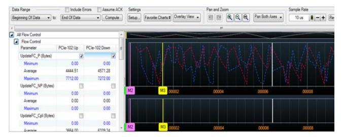
In the above screen, graphs for the Update\_FC\_P series (represented by dotted lines) in both directions are displayed. The blue dotted line represents the graph for Update\_FC\_P series in upstream, whereas, the red dotted line represents the graph for Update\_FC\_P series in the downstream direction.
