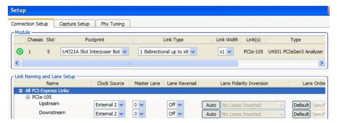
If you have installed multiple U4301A modules in the chassis, all these modules are listed in the Module section of the tab. You need to select the link type individually for these modules.
