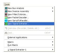
Or, in the Overview window, from a logic analyzer module's drop-down menu, choose **New Tool>Signal Extractor...**.
