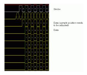
You do not need to rerun Eye Scan, but you run the logic analyzer after each adjustment to verify the results.
