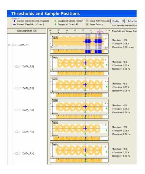
**4** Once the read data sample positions are selected, find the correct sample for the DQS\_R signal. Utilize the waveform view of the state acquisition.
