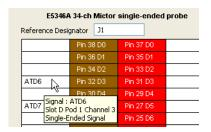
You can clear all FPGA pins that have been mapped to pins/pads by clicking Clear. You can clear individual pin mappings by dragging a pin from the pin/pad diagram back to the FPGA Pins list.
