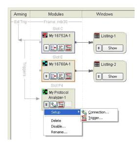
In the next example below, the N5319A correlation cable is used and the logic analyzer sets Flag 3 and then waits for Flag 4 from the protocol analyzer. The protocol analyzer waits for Flag 3 and then sets Flag 4.
