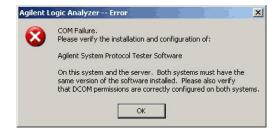
The "Agilent System Protocol Tester" software must be installed on the system where the *Agilent Logic Analyzer* application is running and on the system that is being used as the protocol analyzer server. It can be installed on the logic analysis system frame if you want to run both applications there.
