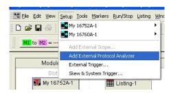
Note that you can set up an external protocol analyzer connection when viewing logic analyzer data *offline* (see Analyzing Correlated Data Offline (see page 29)).
