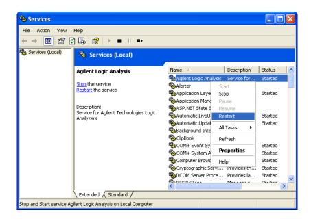
The *Agilent Logic Analyzer* application is taken offline and the service is restarted, which includes the detection of an external 10 MHz CLOCK IN signal. Dialogs and progress bars indicate what is happening. When everything is finished, the *Agilent Logic Analyzer* application is left offline.
