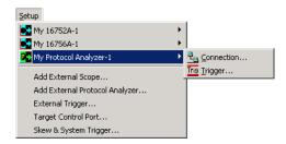
Or in the Overview window, select a command from the protocol analyzer module's drop-down menu.
