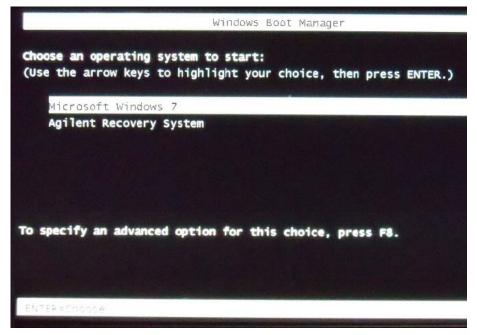
2 After a few seconds, Logic Analyzer automatically starts with the option selected in the Windows Boot Manager. Select the **Agilent Recovery**
