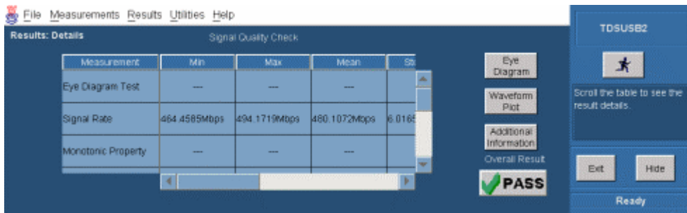
Figure 44: Results details for a High Speed Signal Quality Measurement
