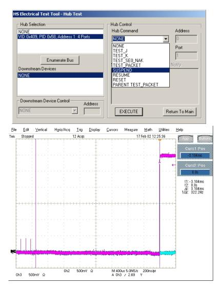
Figure 47: Response to Suspend from Host - Upstream Facing Port
