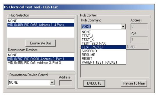
Figure 4: High-speed Electrical Test Tool - Hub Test Menu
