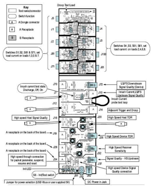
Figure 1: Tektronix New TDSUSBF Test Fixture
