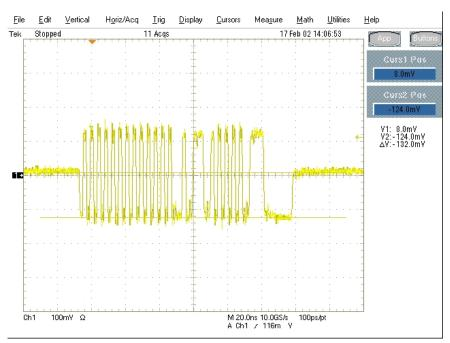
Figure 36: Measuring Differential Voltage Level – Zero to Negative Peak
