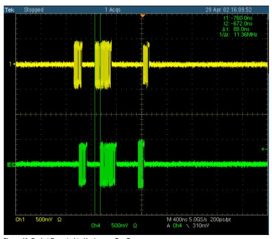
Figure 41: Packet Repeated to Upstream - Top Trace
