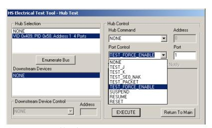
Figure 18: Force-Enable Hub Downstream Port
