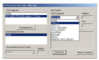
Figure 53: Hub Test\_J from Resume
