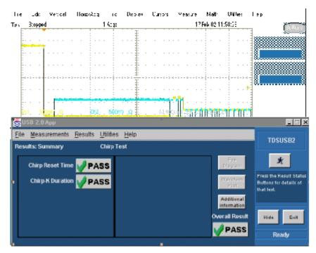
Figure 44: Device Chirp (Speed Detection)
