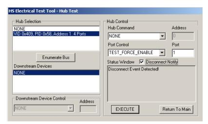
Figure 20: Disconnect Event Detected
