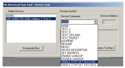
Figure 24: Single Step Set Feature on the Device Downstream of the Hub
