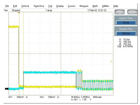
Figure 45: Device Chirp-K Latency
