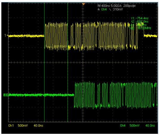
Figure 42: Sync Bit Truncation - No More than 4 Bits
