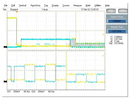
Figure 46: Time From Start of Last J in Chirp K-J-K-J To Device Turns on HS Termination
