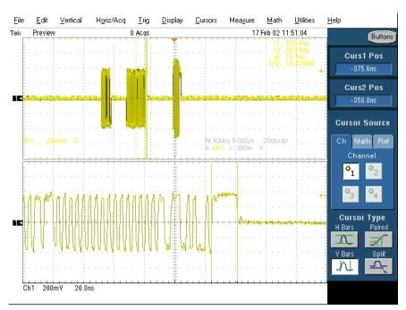
Figure 27: EOP Width - Upstream Packet
