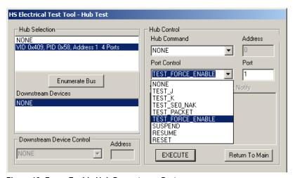
Figure 13: Force-Enable Hub Downstream Port
