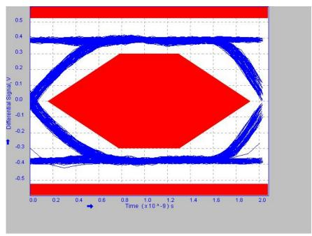
Figure 16: High-speed Near End Eye Diagram
