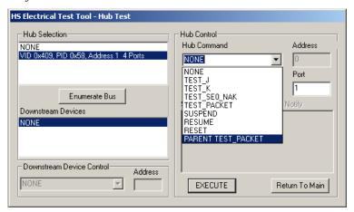
Figure 14: Placing Parent in TEST\_PACKET
