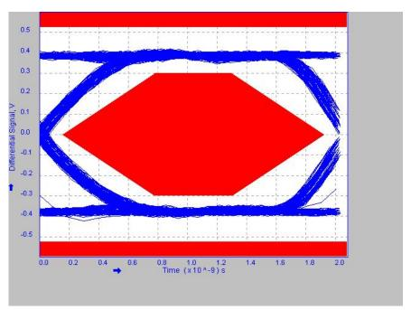
Figure 11: High-speed Near End SQ Eye Diagram
