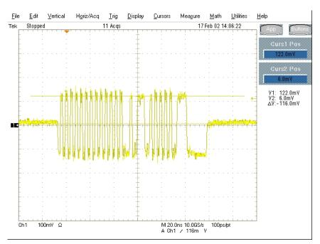
Figure 35: Measuring Differential Voltage Level - Zero to Positive Peak
