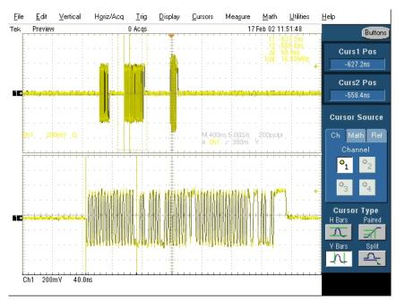
Figure 26: Sync Field Width - Upstream Packet
