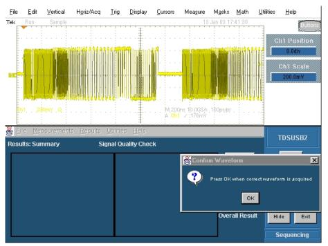
Figure 6: Test Packet from Device
