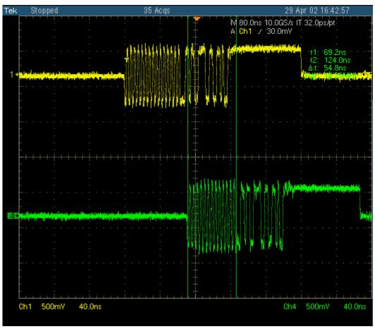
Figure 39: Sync Bits - Downstream Facing Repeater
