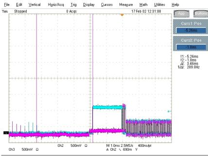
Figure 49: Hub's Chirp-K in Response to Reset from High-speed
