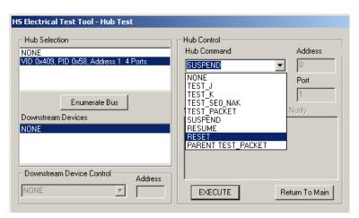
Figure 51: Hub Reset From Suspend
