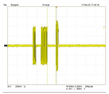
Figure 28: Inter-Packet Gap - Transmit after Receive
