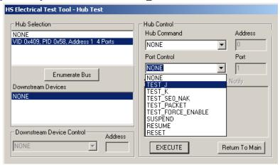
Figure 54: Hub Test\_J
