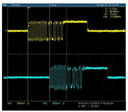
Figure 38: Packet Delay - Downstream Facing Repeater
