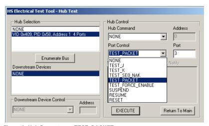
Figure 9: Hub Downstream TEST\_PACKET
