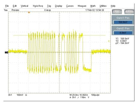
Figure 33: Measuring Differential Voltage Level – Zero to Positive Peak
