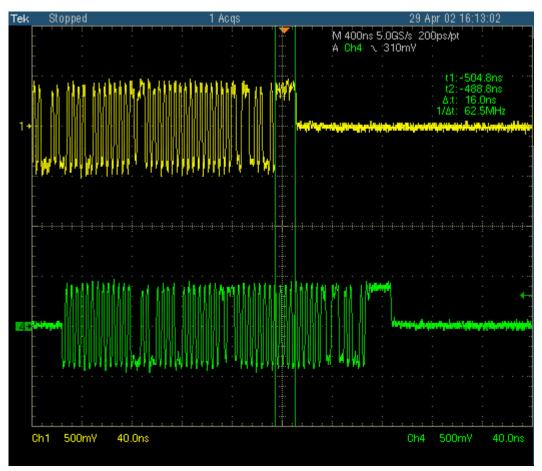
Figure 43: EOP Width - No More Than 4 Added Bits
