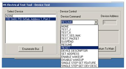
Figure 23: Device Reset
