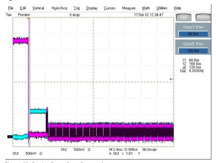
Figure 27: Device Reset from Suspend
