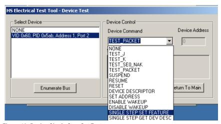
Figure 10: Device Single Step Set Feature
