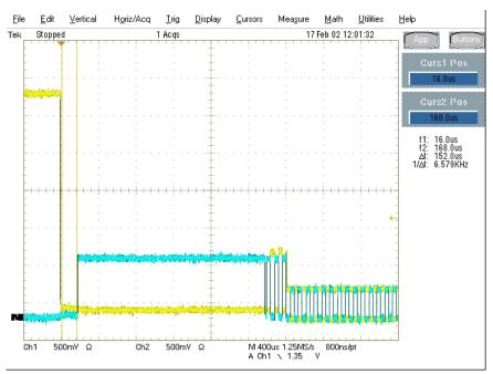
Figure 17: Device Chirp-K Latency
