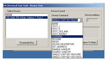
Figure 25: Device Suspend
