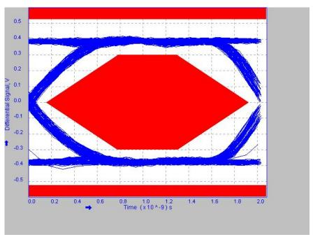
Figure 7: High-speed Near End SQ Eye Diagram
