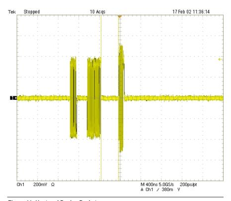
Figure 11: Host and Device Packets
