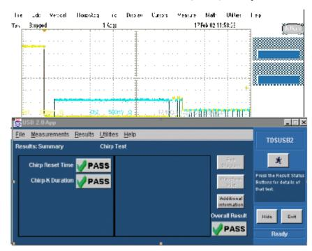
Figure 16: Device Chirp (Speed Detection)
