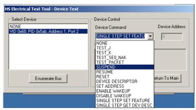
Figure 19: Device Suspend
