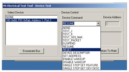
Figure 26: Device Reset
