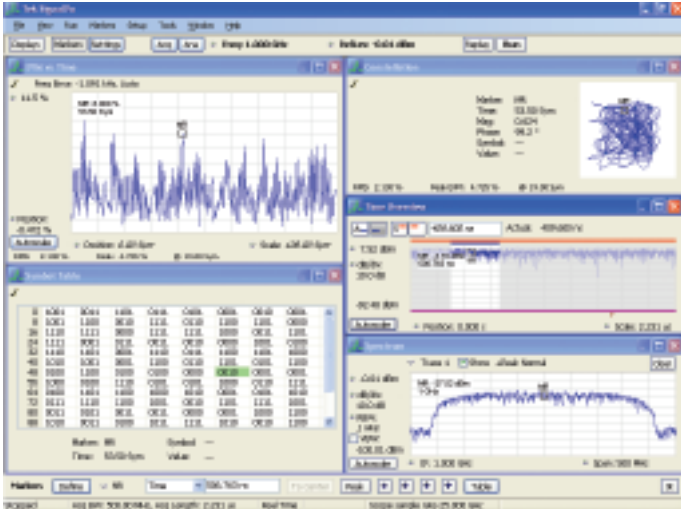
Figure 6. Wideband point-to-point microwave links can be easily demodulated with SignalVu’s option SVM. Shown is a 16QAM signal operating at 312.5 Msymbols per second. Note the RMS EVM of less than 3%.
