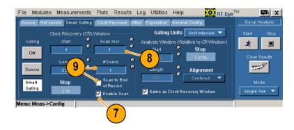
**Setting up the Analysis Window.** After setting up the Clock Recovery Window, you must set up the Analysis Window. There are three ways to set up the Analysis Window.
