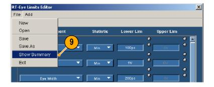
The summary table displays all the measurements, statistics, lower limits, and upper limits that you have set up.
