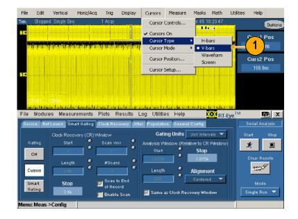
In the application menu bar, select Measurements > Configure > Smart Gating.
