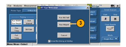
If the RT-Eye Welcome dialog box does not display, select Measurements > Wizard.... File Modules Measurements Plots Results Log Utilities Help RT-Eye<sup>TM</sup> M X Select Configure Start 4 Limits × Jitter @ BER Wizard. Eye Width/ Eye Height Emphasis Run MyTest 123 Select Plots Rise Save MyTest TIE Jitter rude Time жтр Low Amplitude Mode Fall Time nu: Meas->Select
