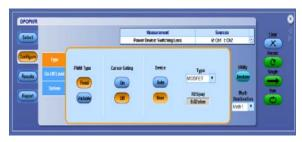
Select the source (Channel, Math, or Ref) and assign the Voltage and Current channels.
