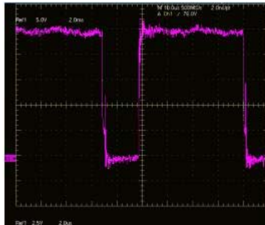
Figure 24: Gate signal without a glitch
