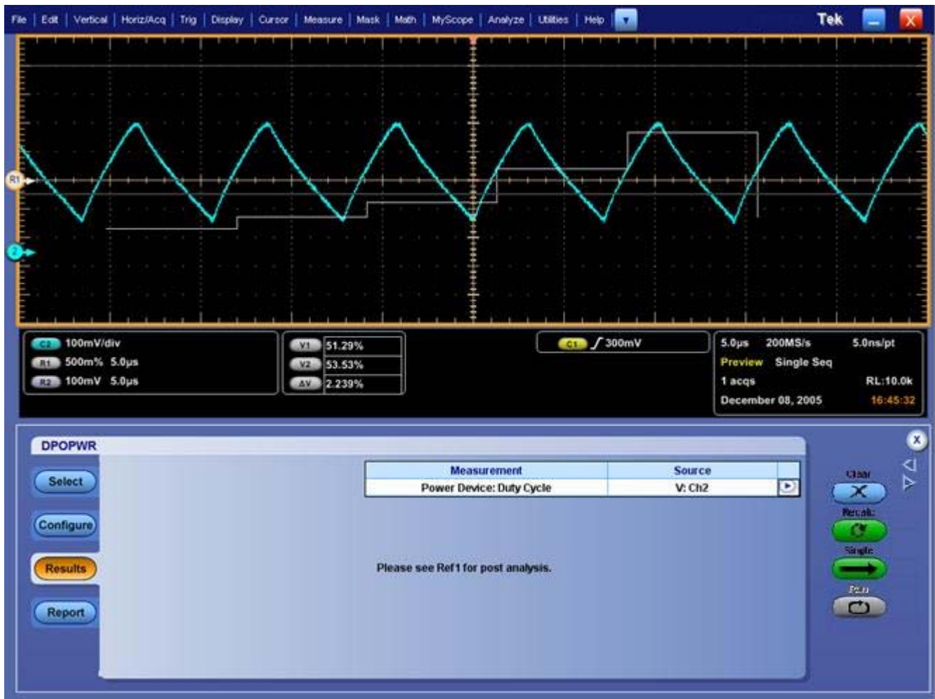
Figure 39: Duty cycle modulation results
