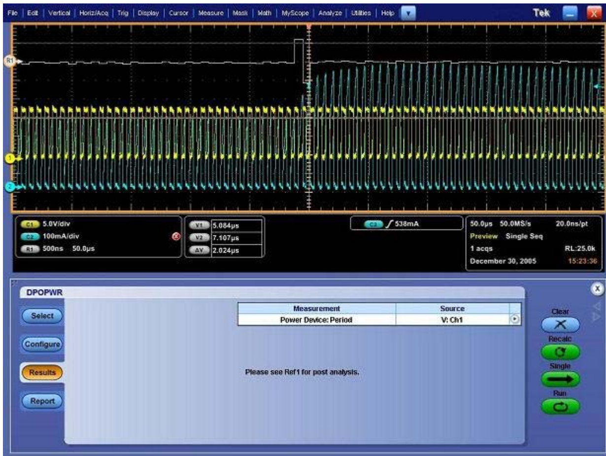
Figure 41: Period modulation results
