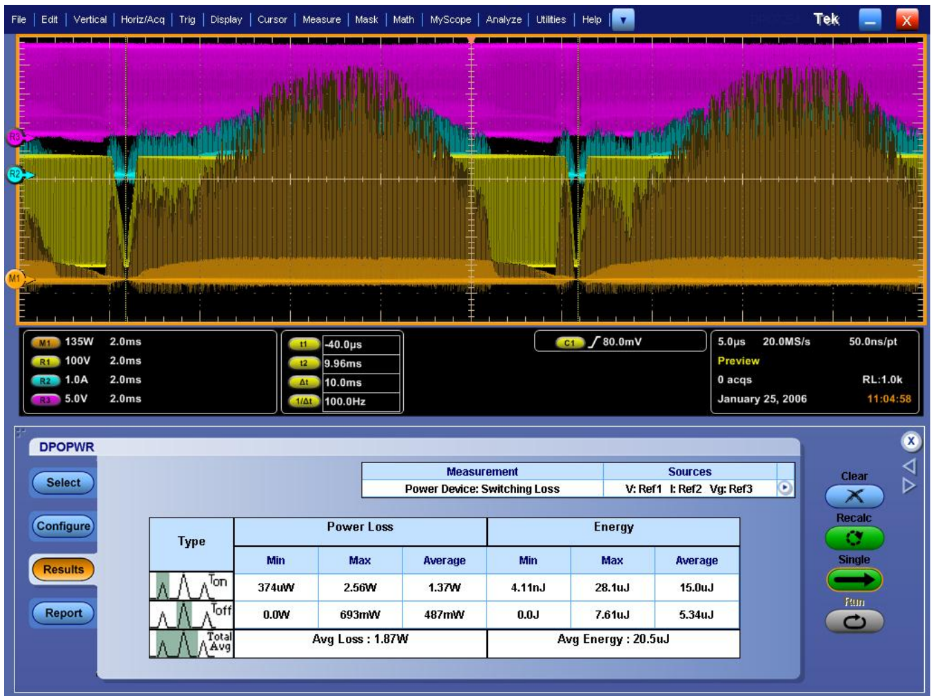
Figure 98: Switching Loss Results
