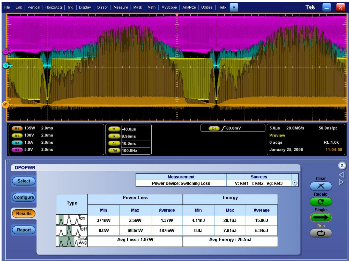
Figure 21: Switching Loss results
