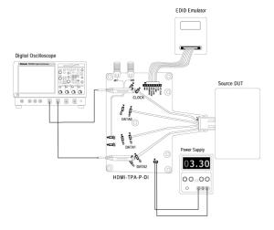
6. Ensure that your signal in the oscilloscope display is similar to the sample signal. Click View Waveform to display a sample of the expected signal. If the displays are not similar, go back and check your configuration and connections.
