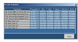
The software calculates statistics for each selected test, and logs the statistics on a cycle-by-cycle basis in a fairly large waveform. The standard statistics are for the Maximum, Minimum, Mean, Standard Deviation, and Population.
