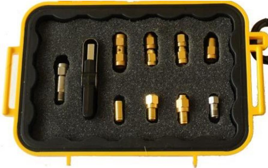
The page gives you the information needed to use the SMA calibration and verification kit on the following **HP** or **Agilent** VNAs.
