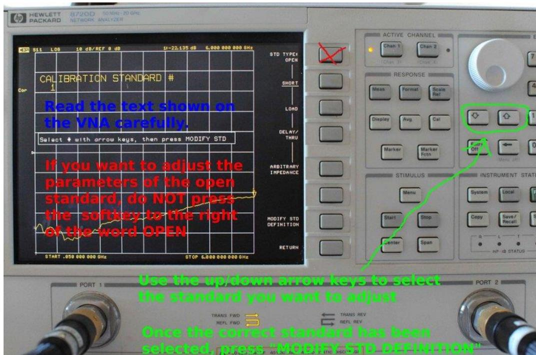
Note in yellow the VNA indicates calibration standard 1. Note that SHORT is underlined. If one wishes to change the parameters of the open standard, it is tempting to press the soft key to the right of the
