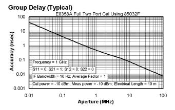
In general, the following formula can be used to determine the accuracy, in seconds, of a specific group delay measurement:
