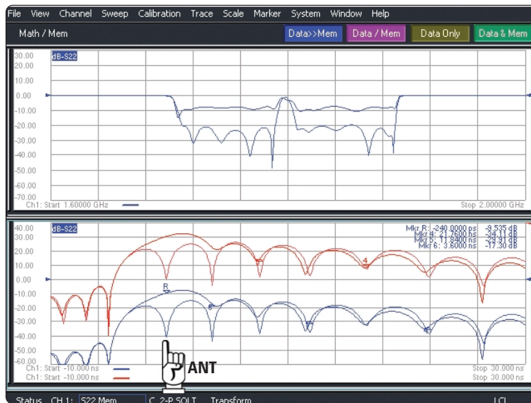
Figure 14. Tuning the common ANT resonator shows a response change primarily in the first null. In this way the first node resonator is determined and the first node frequency can be found by changing the VNA frequency to find the deepest null
