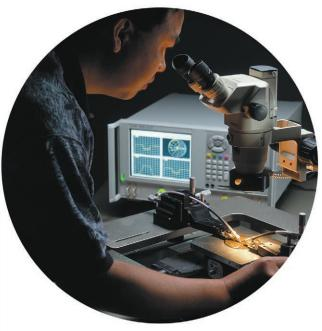
Use TRL calibration for accurate in-fixture or on-wafer measurements.
