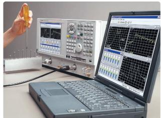
For manufacturers of high-performance bandpass filters, Agilent's new N4261A filter tuning software is the only solution that allows inexperienced filter tuners to rapidly tune multiple-pole filters after only brief instruction. Agilent's filter tuning software is the industry's first complete solution that helps manufacturers reduce average filter alignment times and significantly reduces personnel training times. For more information visit **www.agilent.com/find/fts**
