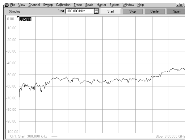
Figure 11. Measurement of load standard after calibration
