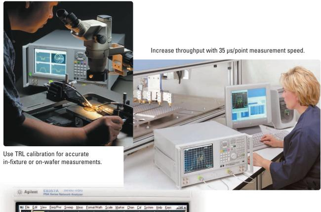
Measure base station filters or LNA/receive filter combinations with up to 143 dB dynamic range.
