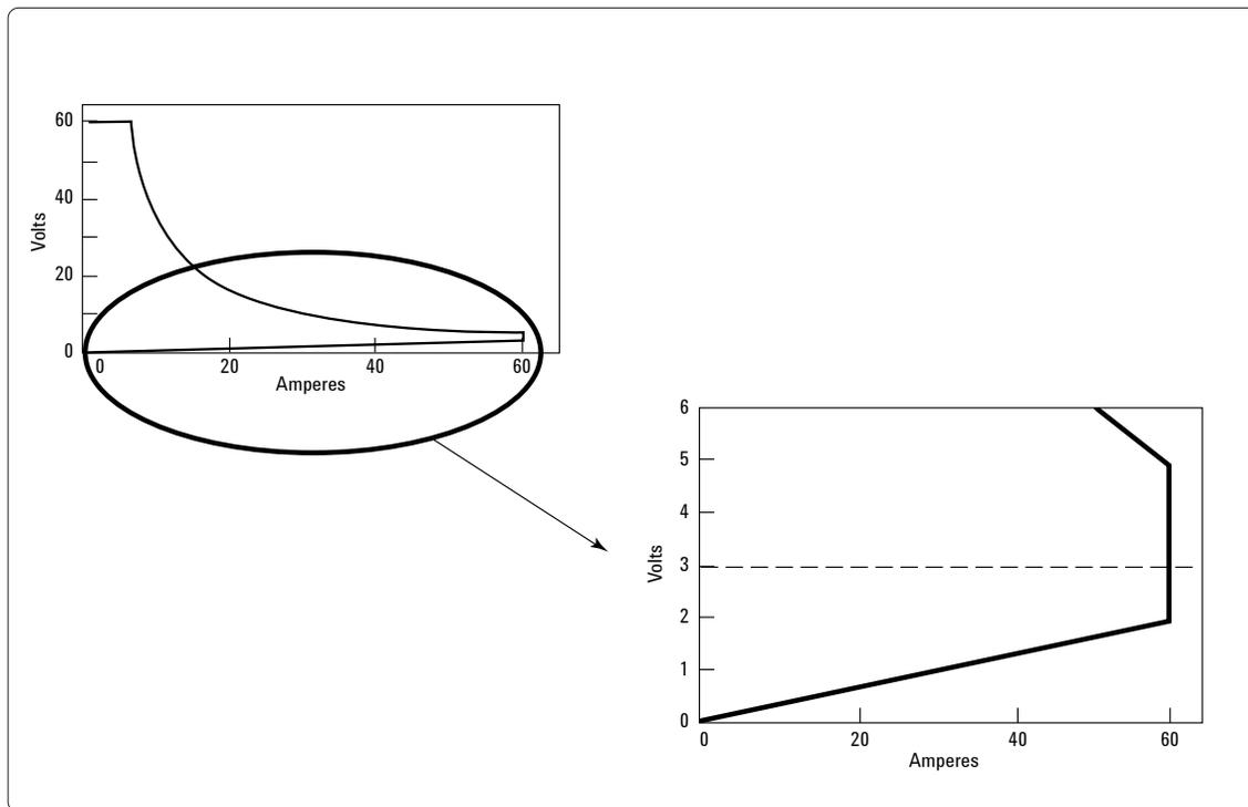
Figure 8. Operating Characteristics of an Agilent Electronic Load
