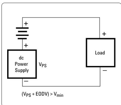
Figure 7. Using an Offset dc Power Supply
