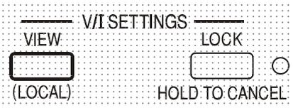
The set voltage and current limit are always shown when the output is off but can also be viewed when the output is on by pressing the VIEW key; the SETTINGS indicator is lit whilst the VIEW key is pressed.
