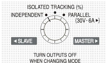
The four operating modes of the Quad-Mode Dual are described below; the mode is changed using the MODE rotary switch. To prevent unintended voltages being accidentally applied to the circuits connected to the outputs, changing modes will always cause both outputs to be switched off.
