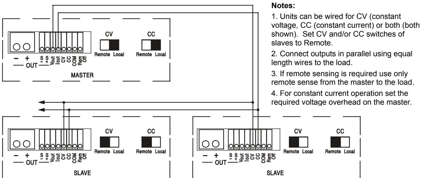
4 In constant voltage mode the voltage across the load is that set on the master unit by its front panel controls, via the digital interface or by the analogue CV remote control input. The current limit for the system (i.e. the current in constant current mode) is the current limit set on the master  $\times n$ , where  $n$  is the total number of units connected in parallel.
