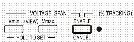
Ratio Tracking is enabled by pressing the ENABLE key in the Slave VOLTAGE SPAN section (ENABLE lamp on)
