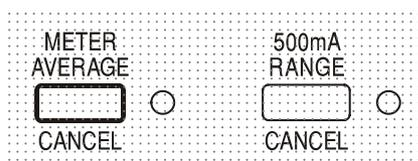
To reduce the measurement jitter with rapidly varying load currents a 2-second time constant can be selected by pressing the METER AVERAGE key; the indicator beside the key lights when meter averaging is selected. Press the key again to CANCEL meter averaging and return to the standard 20ms time constant.
