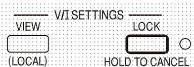
If the output is still on, **OP on** (output on) will flash twice in the display, followed by flashing of the new 'unlocked' settings for 2-3 seconds (slowly at first, then faster) before the change is finally implemented; the LOCK lamp goes off when the change is made.
