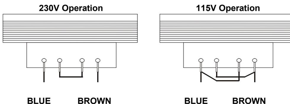
4. Re-assemble in the reverse order. To comply with safety standard requirements the operating voltage marked on the rear panel must be changed to clearly show the new voltage setting.
