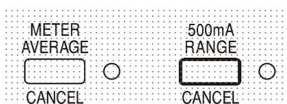
The upper limit of the CURRENT control can be switched between the maximum for this model and 500mA with alternate presses of the 500mA RANGE key to give finer current limit setting and measurement resolution (0.1mA up to 500mA); the indicator beside the key is lit when the 500mA range is selected.
